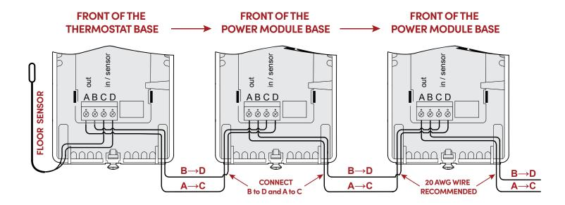
Caution: If the primary and seccondary relays are connected incorrrectly, the secondary relay will be cconstantly pulled. - The floor might overheat
