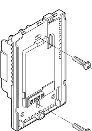
Install the power base into the electrical box.
