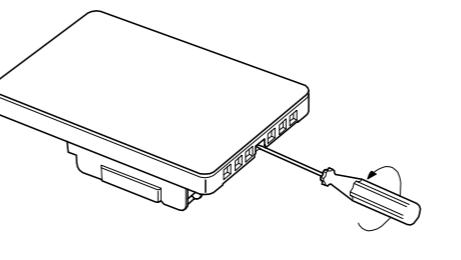
Loosen the screw at the bottom
