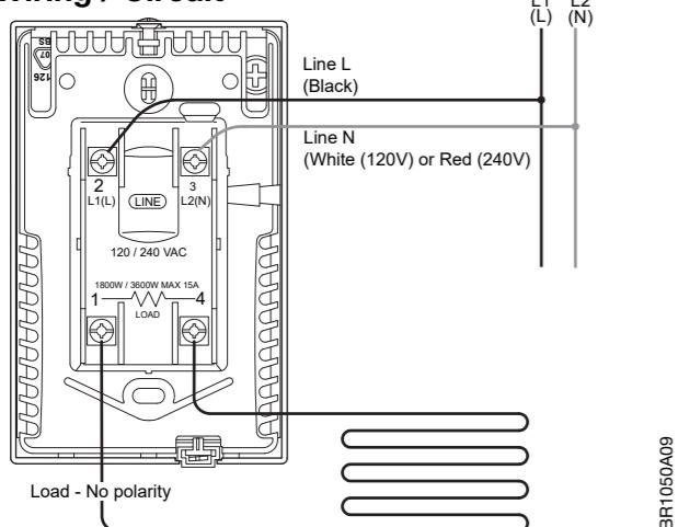
Turn power source OFF at breaker panel. Connect power supply wires to line side and heating cable wiring to load side of power base. AWG between 12 - 20.
