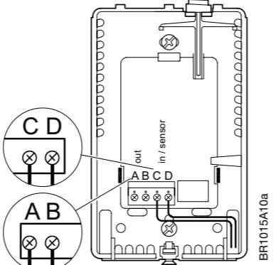
The floor sensor cable must be routed to the junction box separate from power wires and the heating cable cold lead. Ensure that the insulation on the electrical wiring and the floor sensor inside the junction box are not damaged. Thread the floor sensor cable through the hole in the power base. Push the electrical wires to the back of the electrical box.
